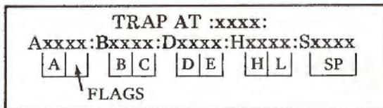
The first line shows the memory location of the RST 7 calling instruction that resulted in the trap routine being called and the second line displays the machine state (accumulator, flags, the registers B,C,D,E,H & L and the stack pointer) at the completion of the last program instruction executed before the trap calling instruction (RST 7) was encountered.
